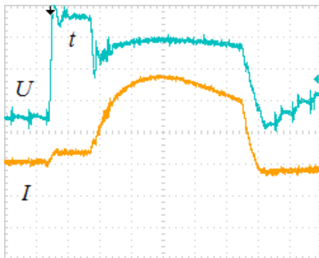
Fig.1. Characteristic oscillograms of the discharge parameters (100 V/div, 50 A/div, 50 \mu\text{s} /div)
