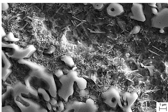
Fig. 1. Microstructure of chrome-vanadium white iron coating after aging.
