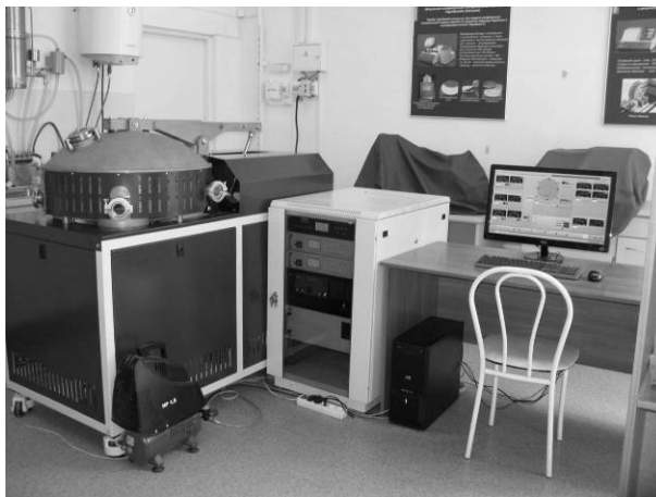
Fig. 1. Universal vacuum setup for RF-magnetron deposition of bioactive coatings on ceramic and bioinert metals.
