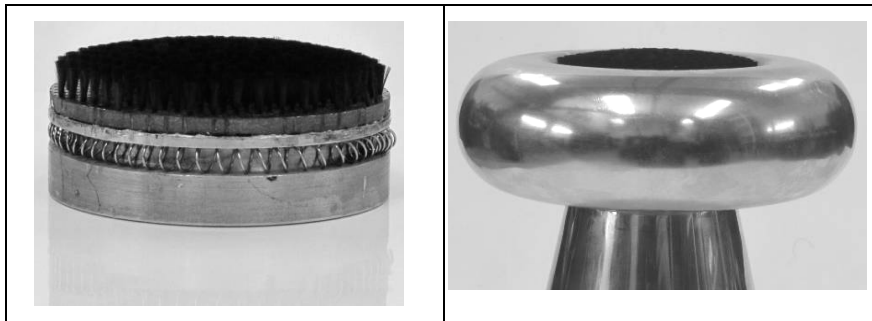
Fig. 1. Fiber carbon cathode (left) and focusing electrode (right)
