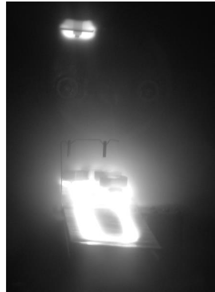
Fig. 2. Photo cathode region of a glow discharge in a magnetic field at a pressure of 80 Pa
